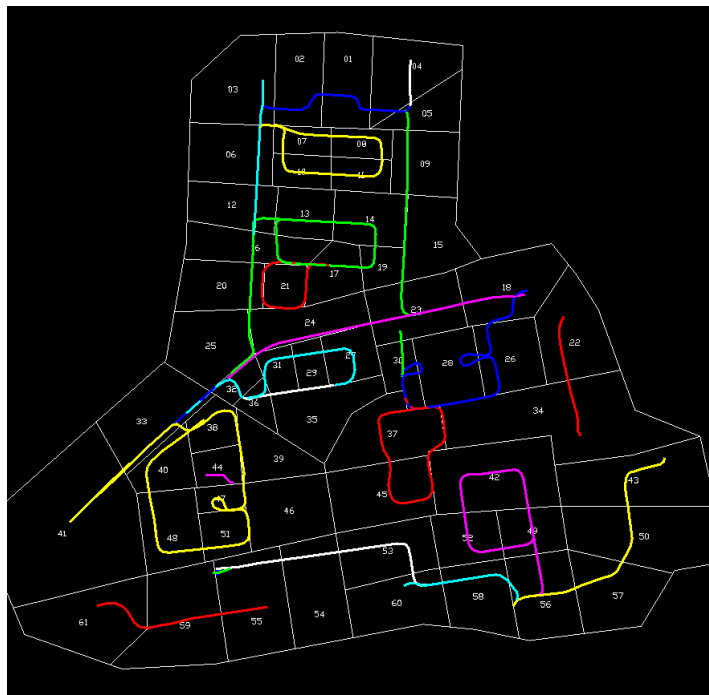
Figure 1. Routes of movement of the system of ground-based laser scanning RIEGL VZ-400 through the territory of 1 MOC and blocks of point arrays
